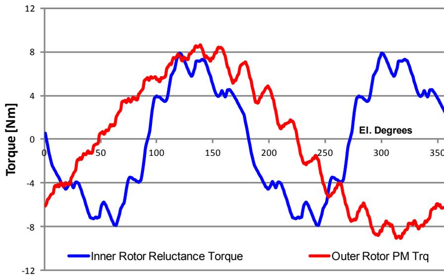
**Fig.3. Dual Rotor LSPM Synchronous Torques**
