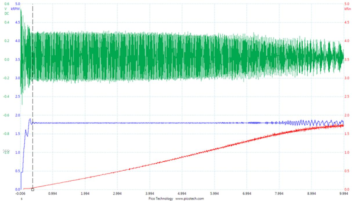
**Fig.7. Dual Rotor LSPM Startup with 4 Nm load with 94 times higher than motor inertia**
