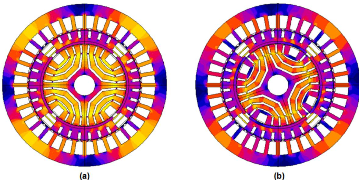
**Fig.2. Flux distribution in Dual Rotor LSPM**
