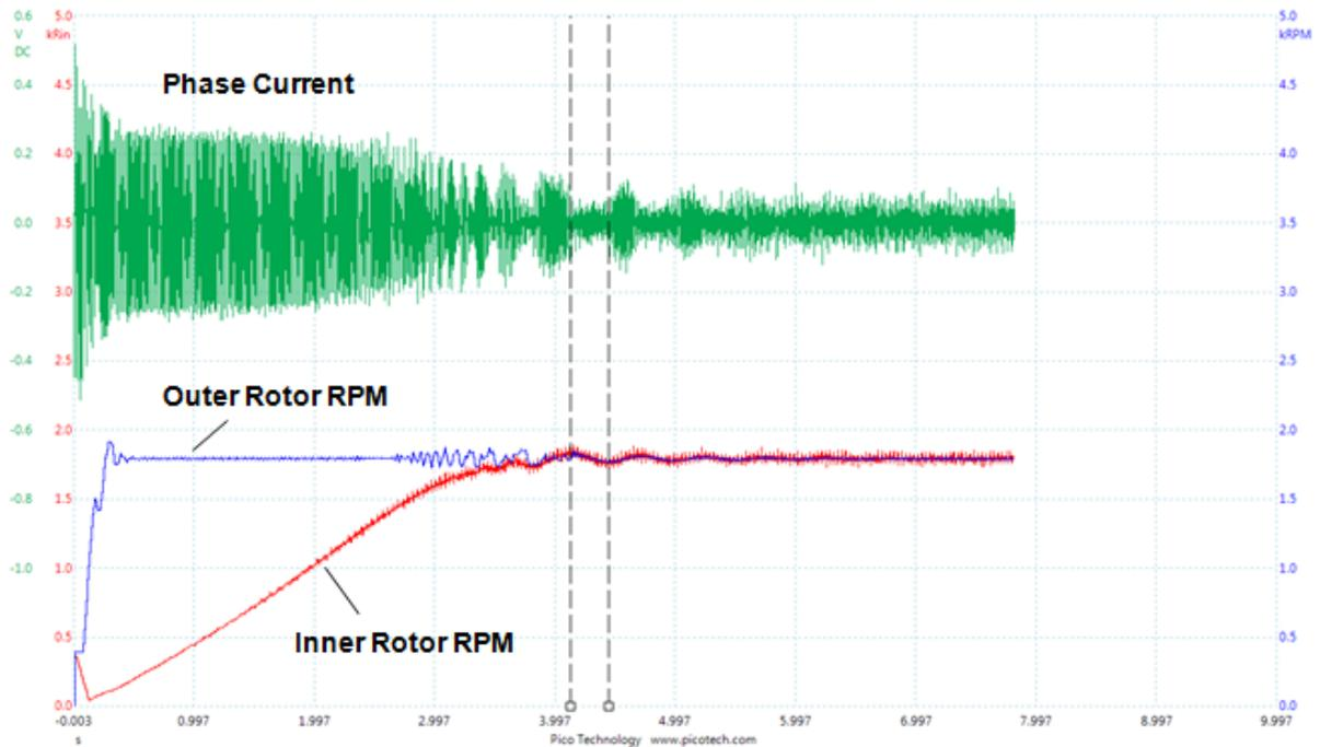
**Fig.6. Dual Rotor LSPM Startup with 4 Nm load with 27 times higher than motor inertia**
