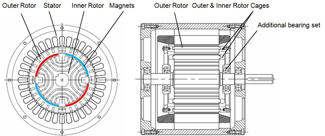
**Fig.1. Dual Rotor LSPM Construction**
