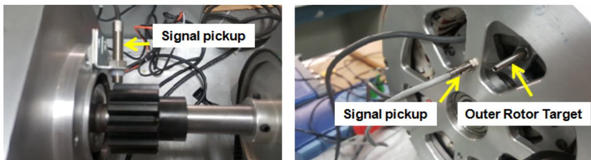
**Fig.4. Rotors RPM measurement**
