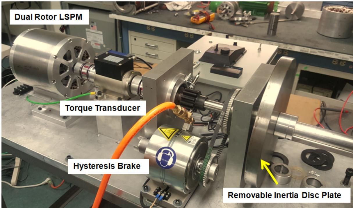
**Fig.5. Dual Rotor LSPM Test Bench**
