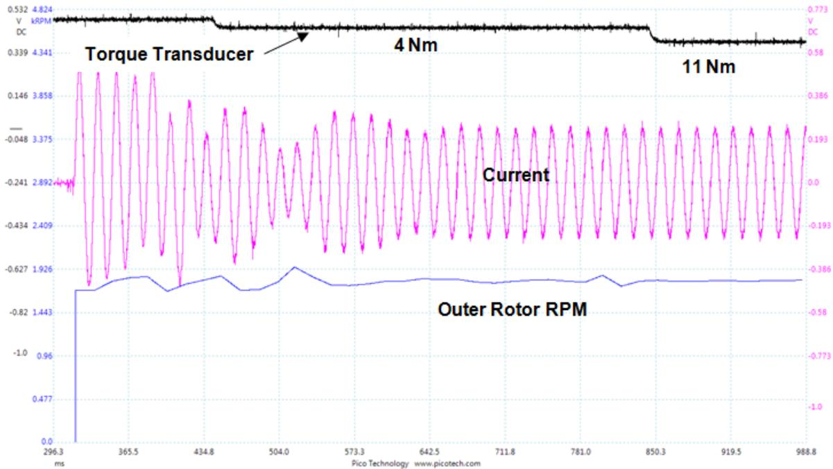
**Fig.8. Dual Rotor LSPM Lock Rotor Test**
